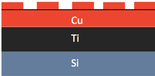
Fig. 5–Top layer of copper in checker board formation
