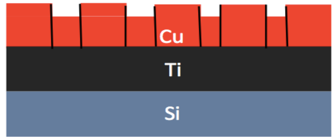
Fig. 6–Layer of copper in checkerboard formation. The copper layer is not partitioned as in Fig. 5.
