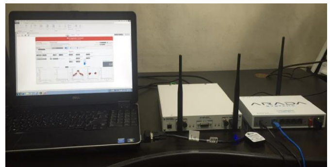
Fig. 1. NI USRP 2943R & ARADA LOCOMATE & LabVIEW Communications with the 802.11 Application Framework.
