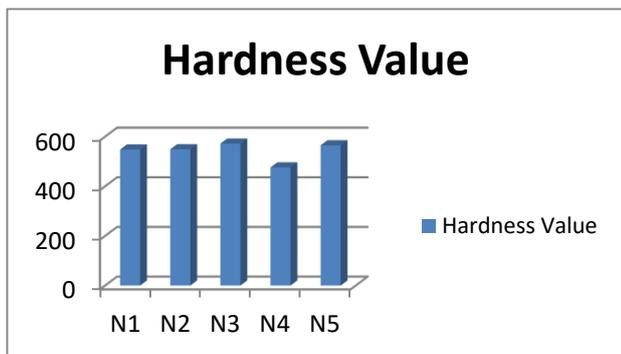
Figure 5: Micro-hardness distributions in the composite coatings
