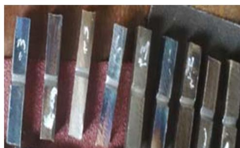
Fig.3. Impact Test Specimen
