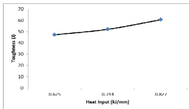
Fig. 8. Plots for Energy input versus Toughness
