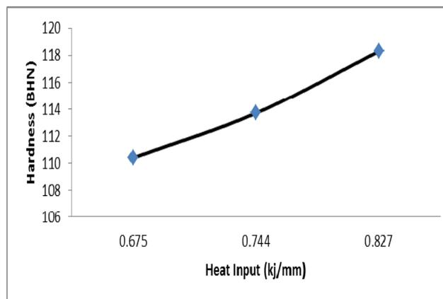
Fig.9. Plots for Energy input vs. Hardness
