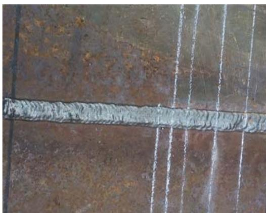
Fig.1. Sample of Butt welded plate using FCAW
