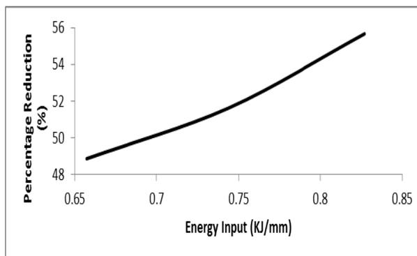
Fig.7. Plots for Energy input vs. percentage Reduction in Area
