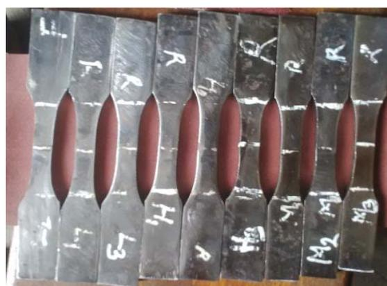
Fig. 2. Diagram of Tensile Test Specimen
