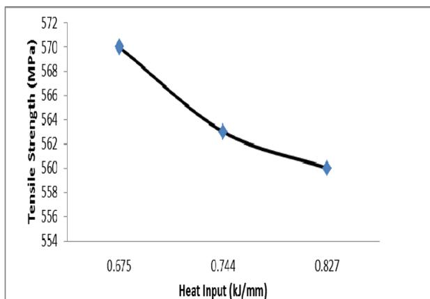
Fig.5. Plot of Heat Input vs. Average Tensile Strength
