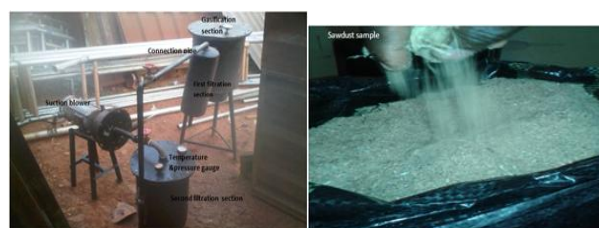
Fig. 4. Picture of the Implemented Gasifier Plant and sawdust
