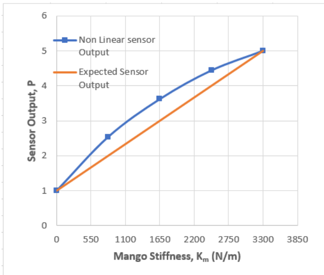
Fig. 8. Nonlinear and Expected Sensor Output Vs Mango Stiffness
